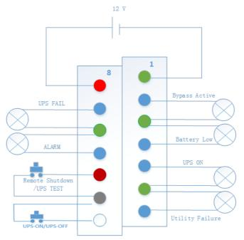
User need to provide power (below 24VDC) and ground. Connect the display and control button to the interface to get UPS operation status and remote shutdown UPS when utility becomes failure.
